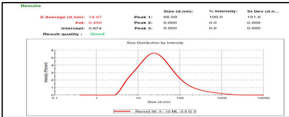
Figure No.5a: It shows that the average nanoemulsion particle size distribution is 19.87nm
